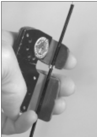
The serving needs to be wrapped counter-clockwise for a left-hand shooter.
