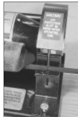
Rotate the shaft to cut around the arrow, not across it.
