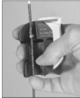
On release, the string rotates clockwise, so the serving should also be clockwise.
