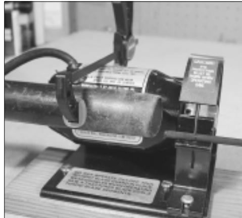
The end of a vacuum hose is clamped to the motor to remove carbon dust.
