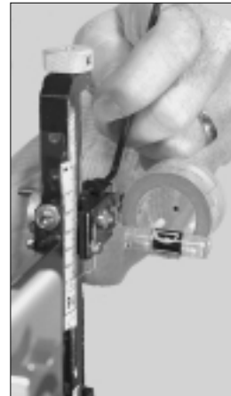
Use the adjustment on the sight block to center the bubble.
